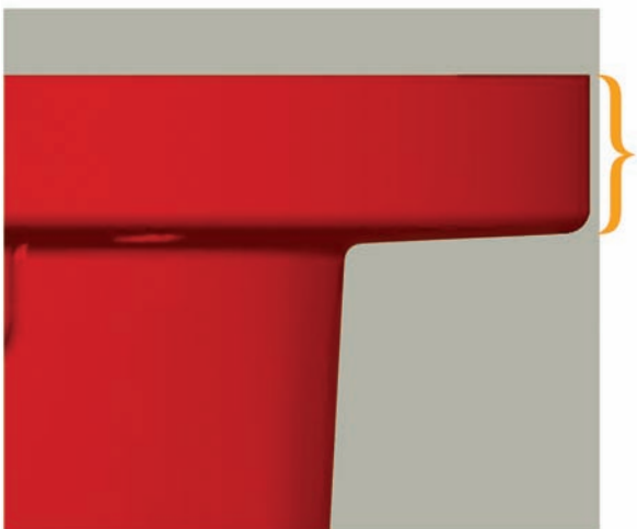
Typical Split-Case 125# Flange Thickness
